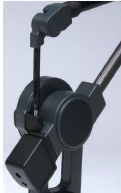
Figure 9 - Correct Home Position for the MicroScribe G2.
