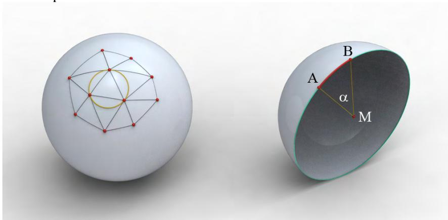
**Fig. 6** Triangulation on a sphere (left). Distances between two points  $A$  and  $B$  can be measured by the associated great circle or the centre angle  $\alpha$ .
