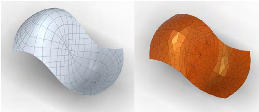
**Fig. 12** The surface  $S$  and a set of its curvature lines (left). The associated planarization with a problematic region in “the middle” of the surface (right)
