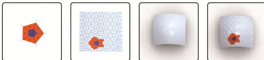
**Fig.1** Ornamental cell, 2D ornament generated with the cell (moving and mirroring), freeform surface and the mapping of the ornament onto the surface
