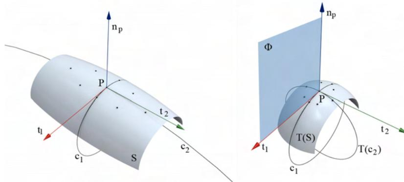
**Fig. 7** A surface point  $P$  with an adapted coordinate system consisting of the principle directions  $t_1, t_2$  and the surface normal  $n_p$  (left). The situation after the transformation  $T$  with the fixed plane  $\Phi$  and the transformed circle of curvature  $T(c_2)$  (right).  $P$  becomes an umbilical point.
