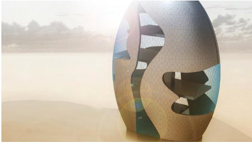
**Fig 13** A smooth double curved surface segmented in plane façade elements
