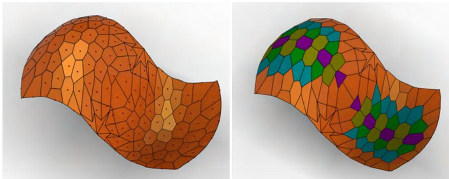
**Fig. 11** The desired spatial version of the ornament shown in Fig. 10 for the complex surface  $S$ . Some of the polygons are colored to enable a comparison with Fig. 10
