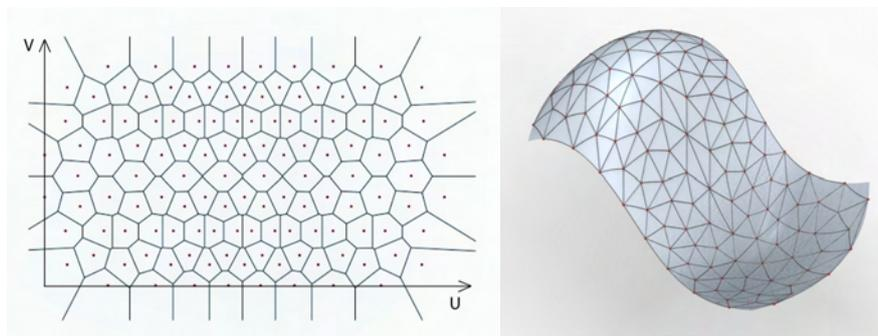
**Fig. 10** A plane ornamental pattern designed as a Voronoi diagram to a certain set of points  $SP$  over the  $[uv]$ -parameter plane (left). Mapping of the point set  $SP$  onto a double curved surface  $S$  and its spatial triangulation (right).
