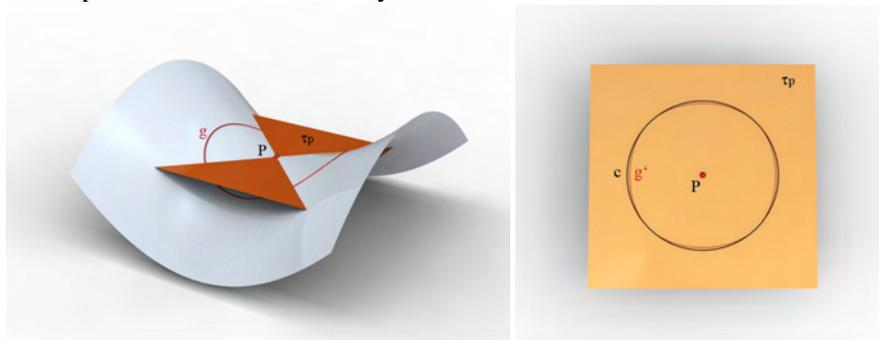
**Fig. 9** A geodesic circle  $g$  with radius  $r$  round the vertex  $P$  of an orthogonal hyperbolic paraboloid (left). Its orthogonal projection  $g'$  into the tangent plane  $\tau_p$  of  $P$  does not differ much from a circle  $c$  with the same radius and the same center  $P$  (right).
