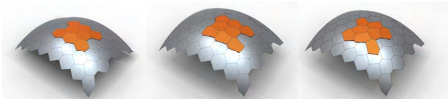
**Fig. 3** Different choices of tangent planes produce different plane panels
