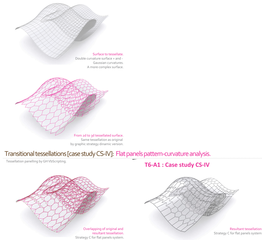
Fig. 5 Figure four shows a non-homogeneous pattern resulting from the iteration between the desired pattern with the combination of both, positive and negative Gaussian curvatures. The output of the ornamental surface, shown in the image, is already enveloped out of flat panels.
